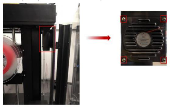
6. Install the Phillips head screws to the back cover.
